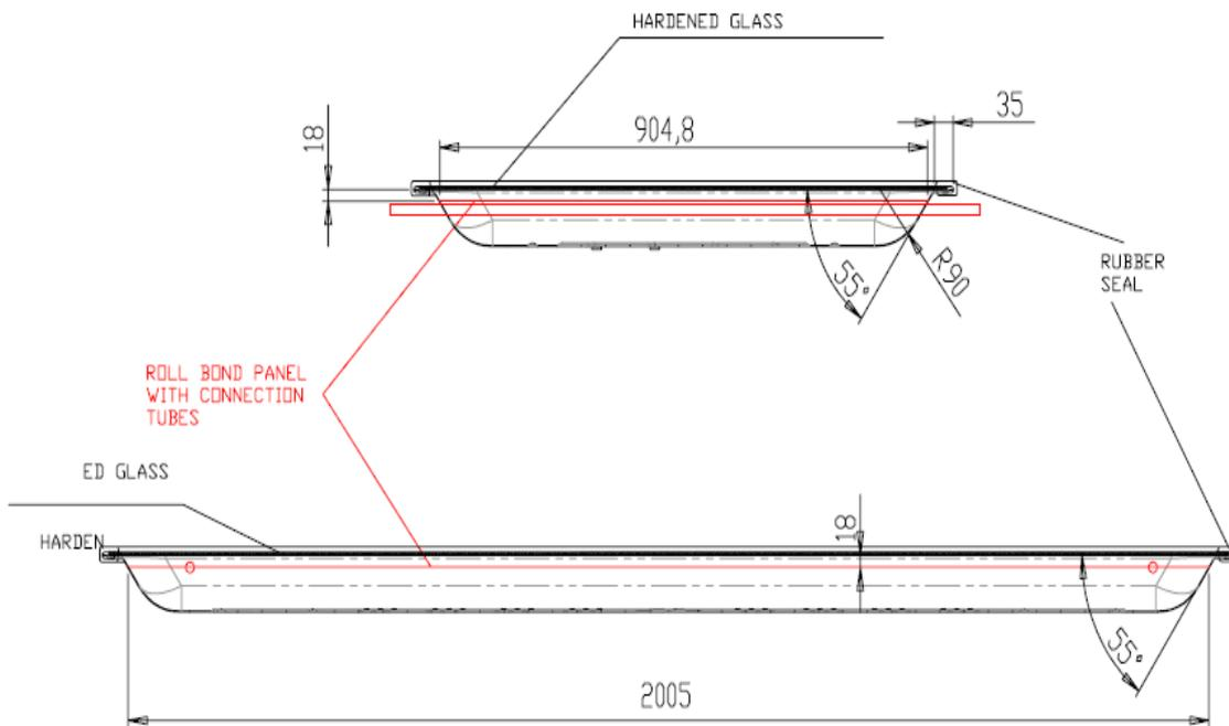
BASIC INSTALLATION ON A SLOPING ROOF FOR THE STANDARD SOLAR SYSTEM COMPOSED OF TWO COLLECTORS.
