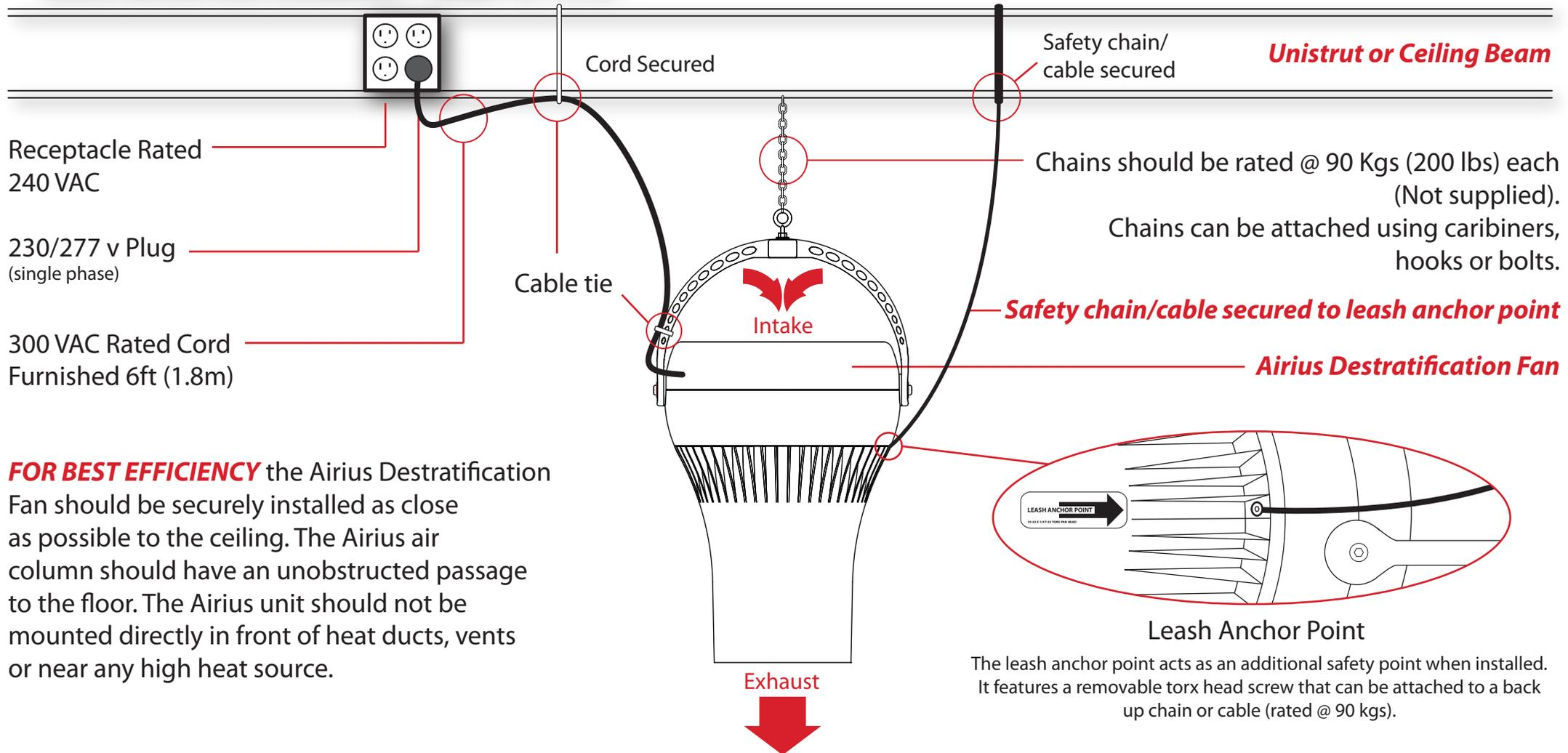
**FOR BEST EFFICIENCY** the Airius Destratification Fan should be securely installed as close as possible to the ceiling. The Airius air column should have an unobstructed passage to the floor. The Airius unit should not be mounted directly in front of heat ducts, vents or near any high heat source.
