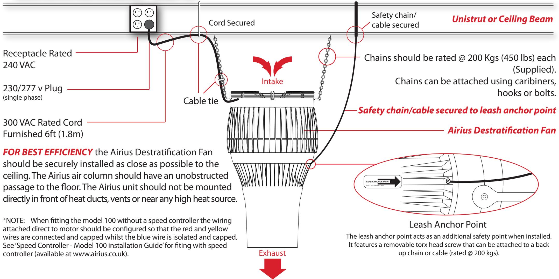
**FOR BEST EFFICIENCY** the Airius Destratification Fan should be securely installed as close as possible to the ceiling. The Airius air column should have an unobstructed passage to the floor. The Airius unit should not be mounted directly in front of heat ducts, vents or near any high heat source.
