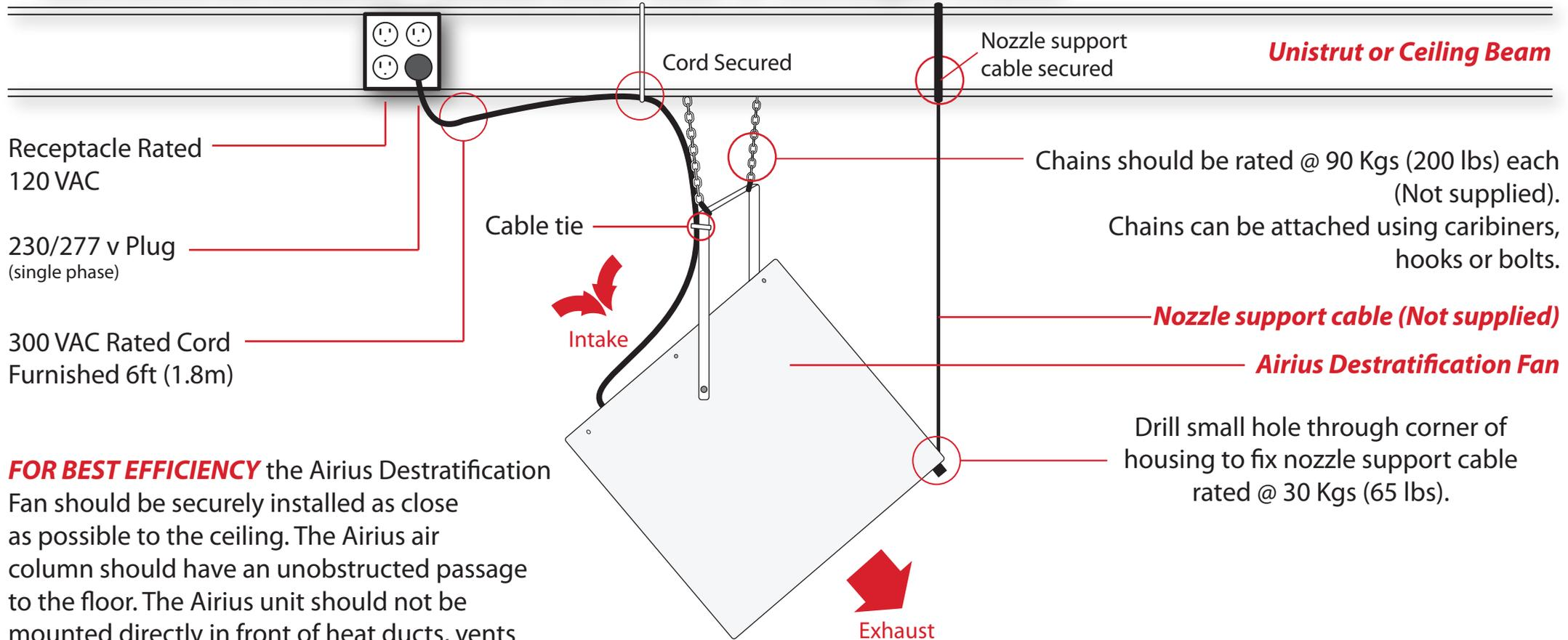
**FOR BEST EFFICIENCY** the Airius Destratification Fan should be securely installed as close as possible to the ceiling. The Airius air column should have an unobstructed passage to the floor. The Airius unit should not be mounted directly in front of heat ducts, vents or near any high heat source.
