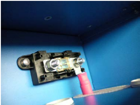
48V battery – single cable Single battery cable to fuse holder 200A fuse
