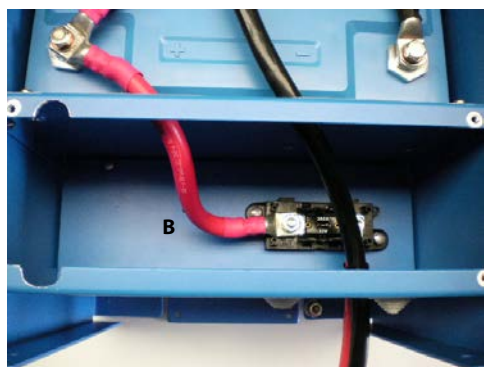
24V battery – single cable For CB battery type place 1x link #B. For BMS battery type make BMS cables connections first before placing this link!
