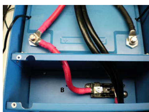
24V battery – double cable For CB battery type place 1x link #B. For BMS battery type make BMS cables connections first before placing this link!
