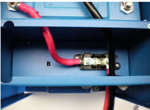
48V battery – single cable For CB battery type place 1x link #B. For BMS battery type make BMS cables connections first before placing this link!
