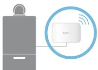
**Extension Kit** to install tado° wirelessly or for boilers without a room thermostat, you will also need the Extension Kit. It connects directly to the heating system.
