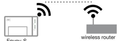
If you are not using the Installer Toolkit mobile app, initiate a WPS connection by pressing and holding the Envoy-S AP Mode button for 5 seconds.
